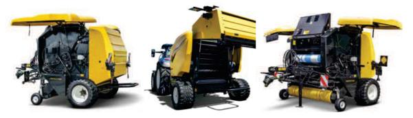
The new Roll-Bar™ 125 fixed chamber Baler produces a bale of 1.25m diameter and is built on the strong heritage and DNA of the best selling BR6000 range. The proven characteristics of simple reliable drive-lines, easy maintenance and high crop flexibility have been improved and enhanced to meet the needs of today's farming operations.
