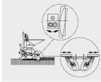
Seed closer with disc is equipped with discs, and canal openers are engaged to each sowing unit which is lined up on a single chassis.
